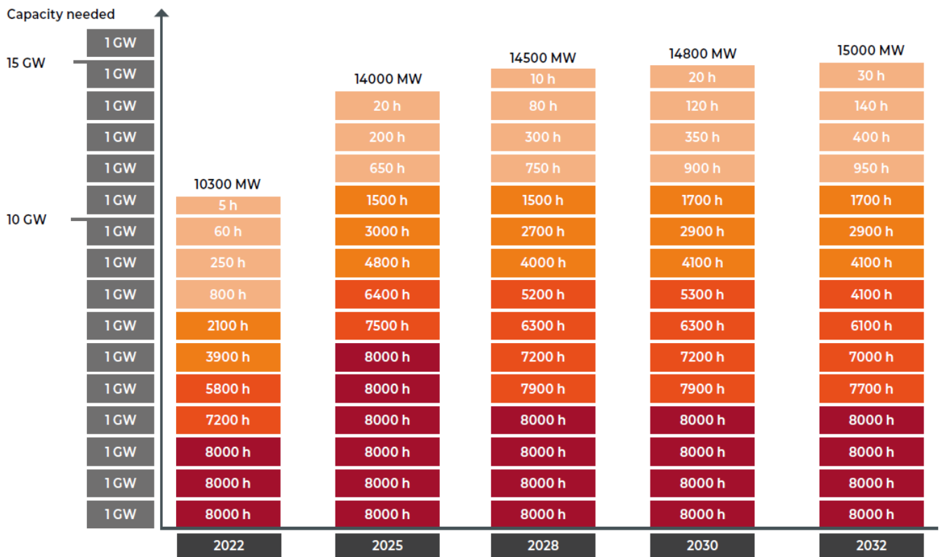
Figure 13 Residual load for Belgium; during how many hours is a certain capacity required, in addition to RES and nuclear capacity according to 'central' scenario, Elia, fig. 5-3, p.166
